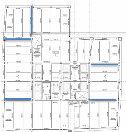
Figure 4 | Location of Composite Beams (S108)
